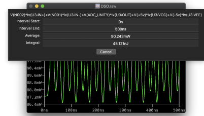
(c) Power dissipation of First ADC OpAmp
