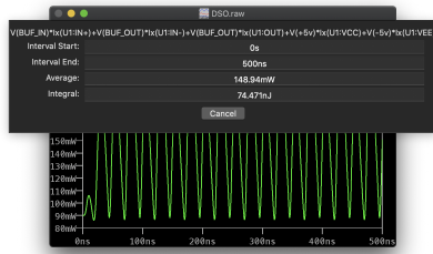
(a) Power dissipation of Buffer OpAmp
